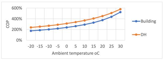
Figure 9: Heat pump COP curves
